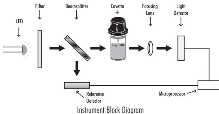
The internal reference system (reference detector) of the [HI97771](#) photometer compensates for any drifts due to power fluctuations or ambient temperature changes, providing a stable source of light for your blank (zero) measurement and sample measurement.
