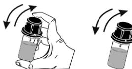
In order to avoid reagent leaking and to obtain more accurate measurements, close the cuvette first with the supplied HDPE plastic stopper
